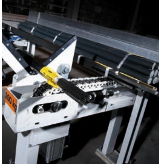
Manual bundle unit with material bundle conveyor (plastic lined).
