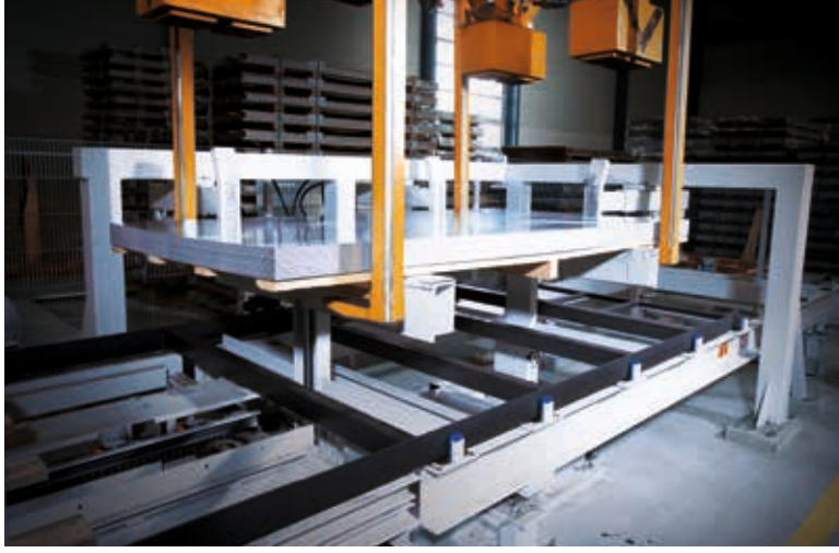
Loading one end of a double deep sheet pallet using a sheet lifter.
