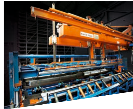
Commissioning unit with vacuum traverse for non-magnetic bar stock.
