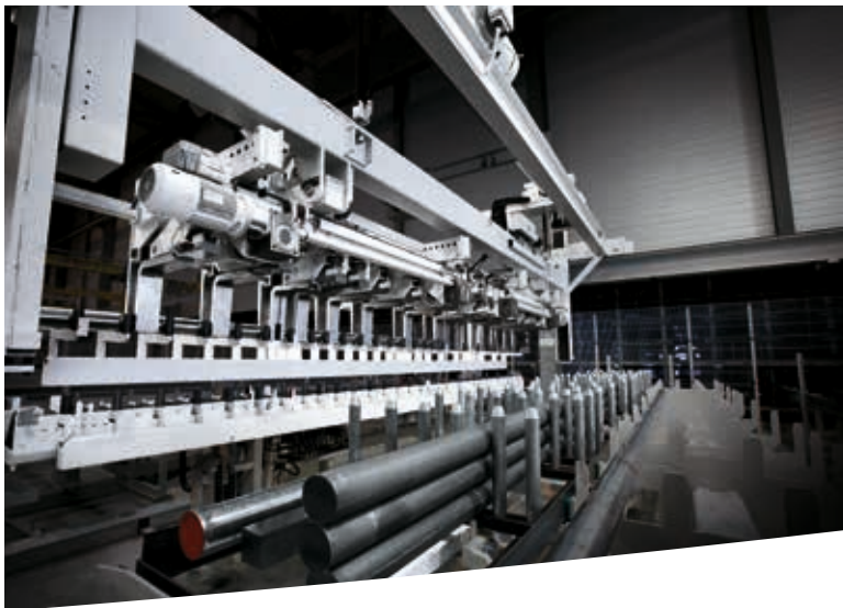
KASTO single bar manipulator retrieving a bar from a cassette from above.
