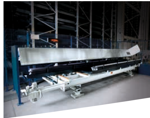
Input station with lift unit and stop portal for easy storage of customer-own bar stock cradles via forklift.
