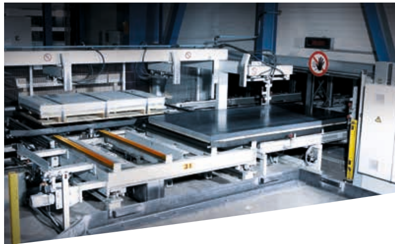
Rotary station with storage table for sheet metal packs to be loaded with forklift or crane.
