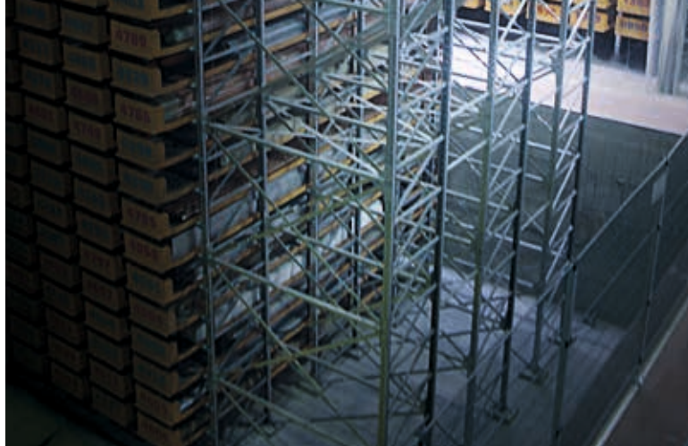
Honeycomb storage system in a pit.
