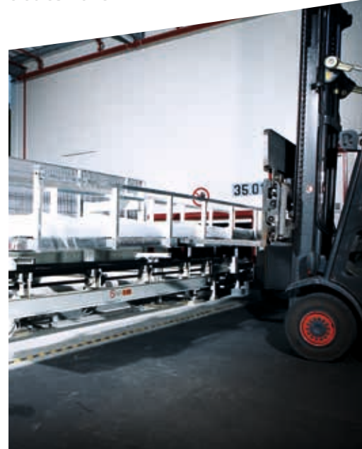
Input station with lift unit and stop portal for easy storage of customer-own bar stock cradles via forklift.
