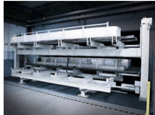
Rotary station at front of storage system with protective cover for cassette change during material removal.
