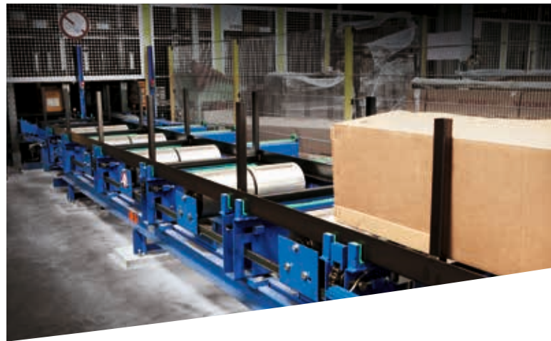
Station with integrated roller conveyor.
