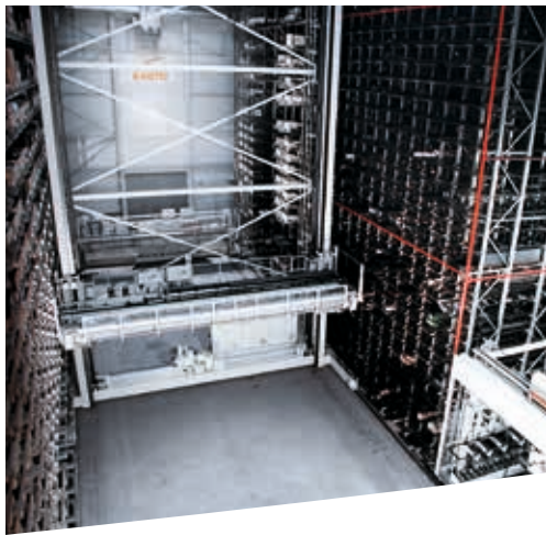
Honeycomb Storage System with saw cell as logistics center for bar stock, sheet metal, Euro pallets.
