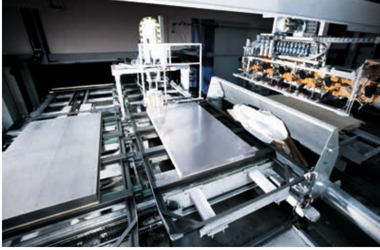
Rotary station with fully automatic sheet metal commissioning.
