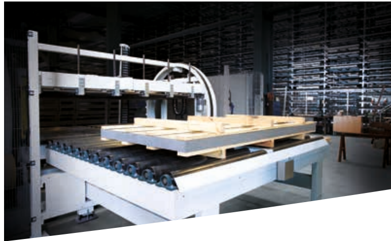
Sheet turning machine for semi-automatic unpacking of sheet metal packs.
