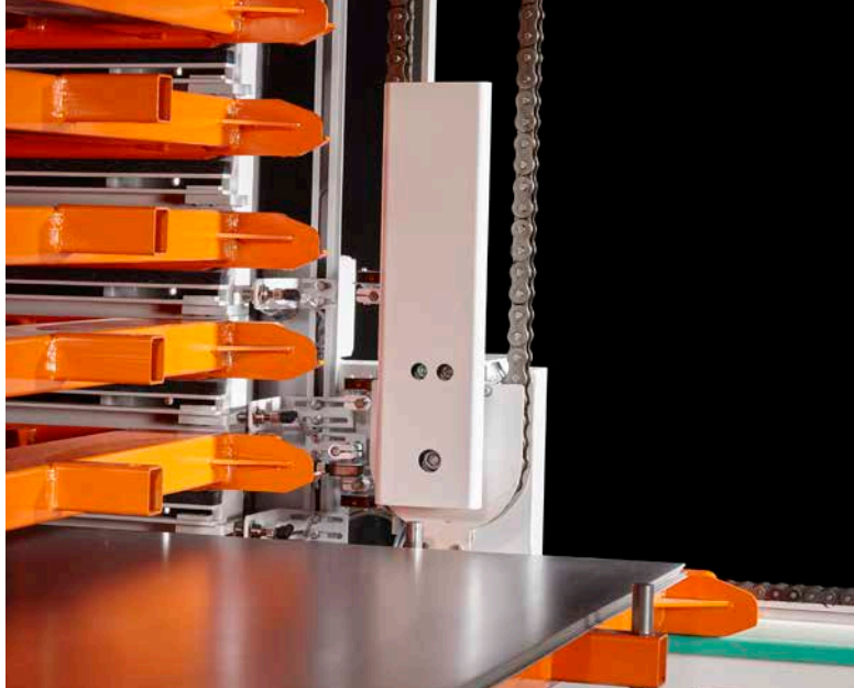
KASTO AdvancedControl storage control with compartment preselection and acknowledgement key Lifting beam and pallet in sheet metal format with chain hoist and loading height control and steel construction with sliding support, pallet with socket pins (option).
