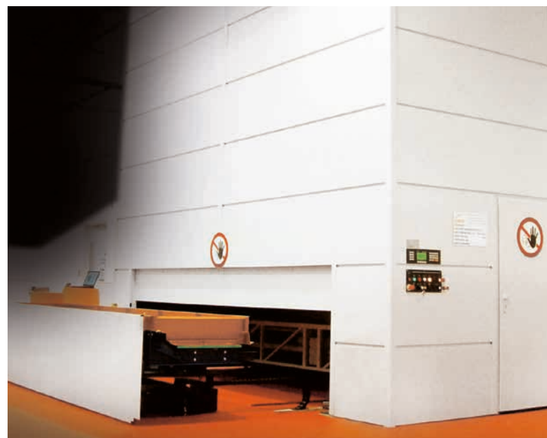
UNITOWER with in-house cladding to protect stored goods
