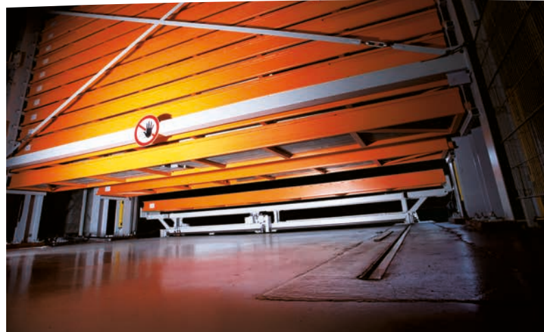
Material tower with material on both sides
