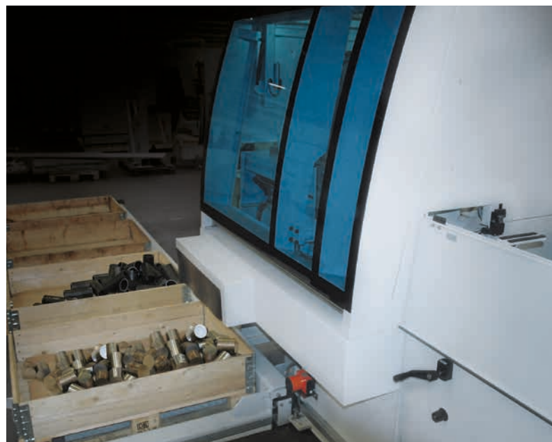
Sorting device with several container locations for cut-off pieces
