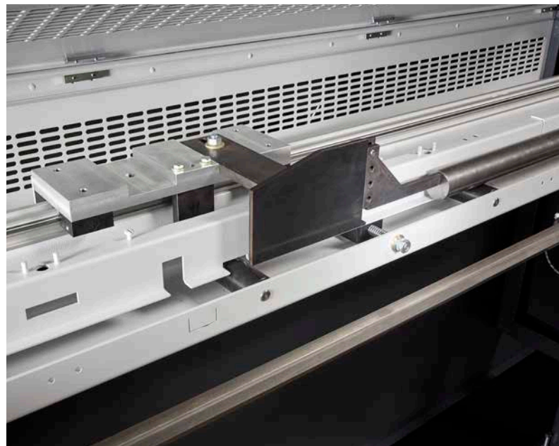
Feed cart with linear guide system and material guide rail
