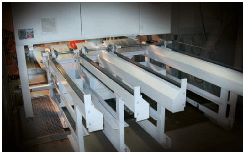
Sorting of long cut pieces inside the machine
