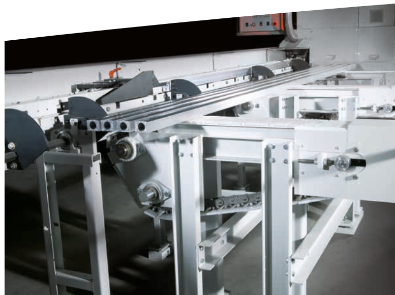
Flat magazine for rectangular and special profiles
