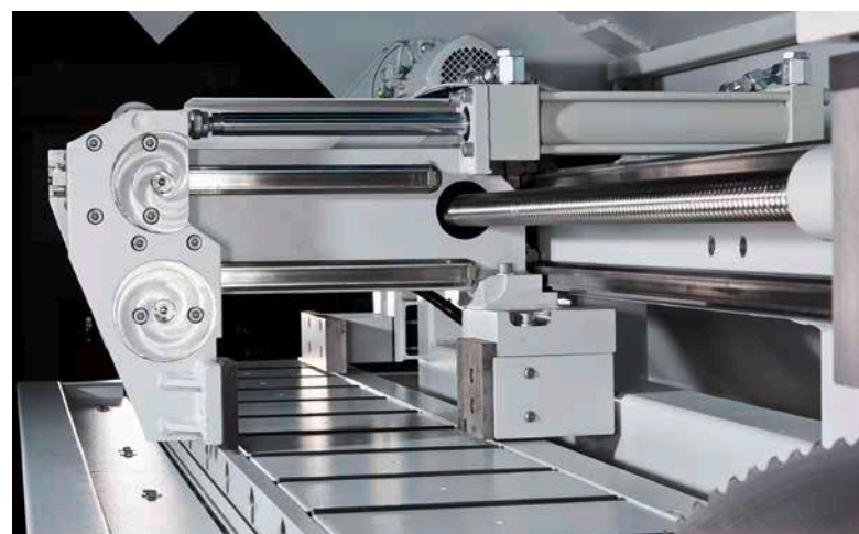
Vice for material feed on KASTOflex A and KASTOflex F
