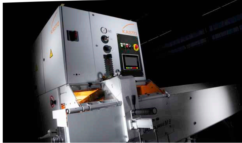
Machine control with technology input via touch screen
