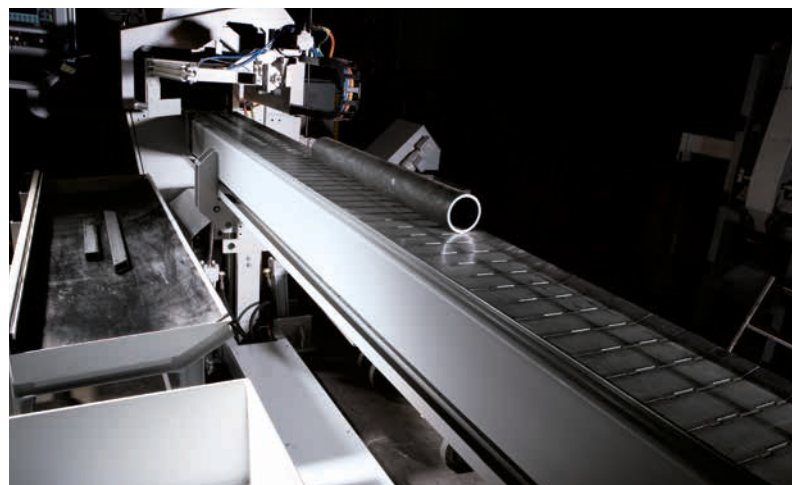
Cut piece sorting plate conveyor for the KASTOflex F
