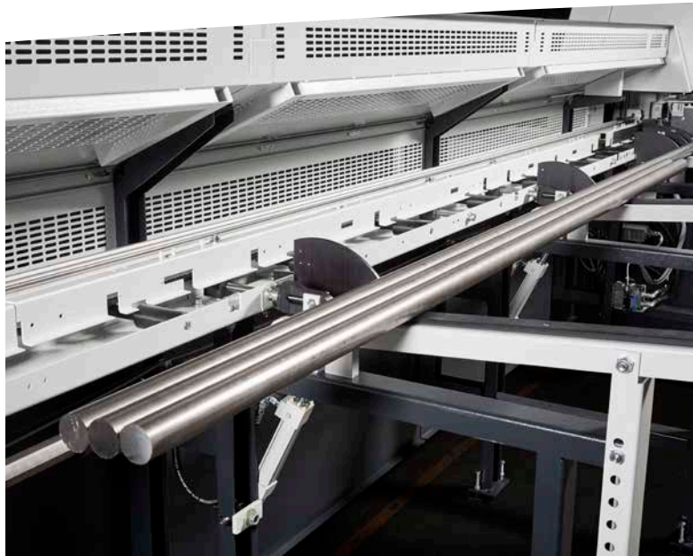
Inclined magazine with loading discs and infeed roller conveyor
