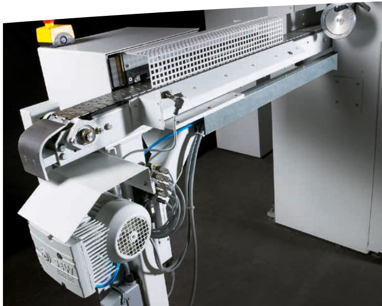
Cut piece outfeed conveyor with sliding device ("to the left" version)
