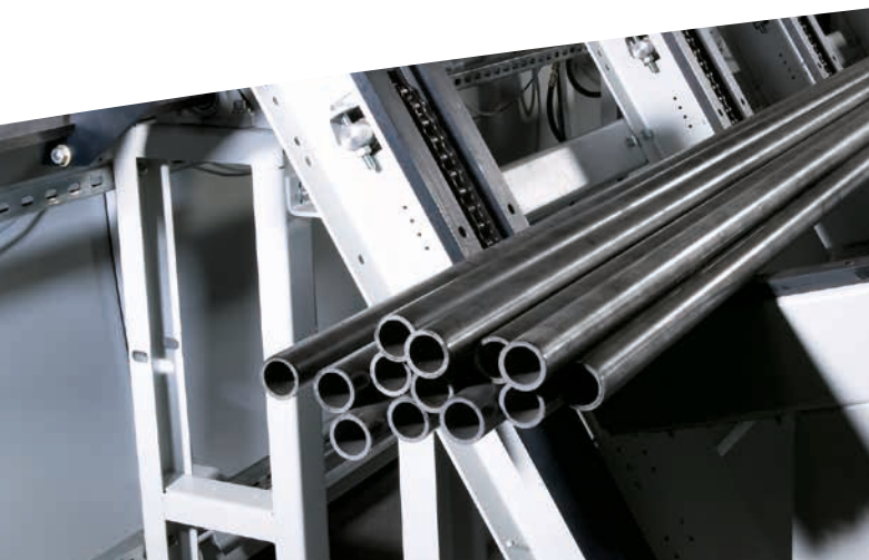
Bundle loader with material in loading position.
