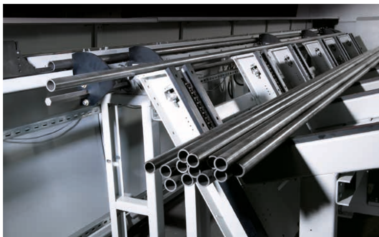
Bundle loader with material in laying position
