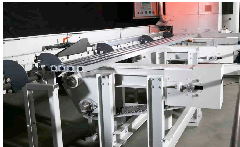
Flat magazine for rectangular and special profiles
